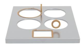
Protect the countertop by placing painter's tape around all openings.
