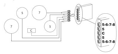
IMPORTANT: Do not lengthen or shorten the wire for any cooking zone, as this will void the product warranty. Tulip Cooking will not be held responsible for any damage, malfunction, or hazard caused by a wiring change done by the customer.
